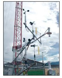
The CR1000 is compatible with the LLAC4 Low-Level AC Conversion Module. Use of the LLAC4 allows more wind sensors to be measured for wind profiling applications. Wind profiling helps customers determine if a site is a good candidate for harvesting wind.
