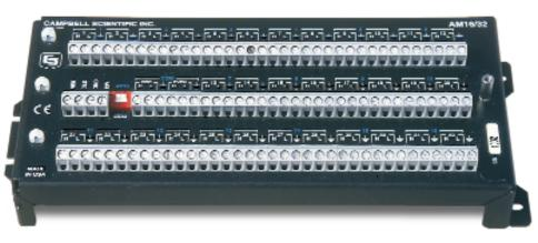
The AM16/32 combines the attributes of our AM416 and AM32 multiplexers. It can be manually configured to multiplex channels in 16 groups (four lines at a time) or 32 groups (two lines at a time).
